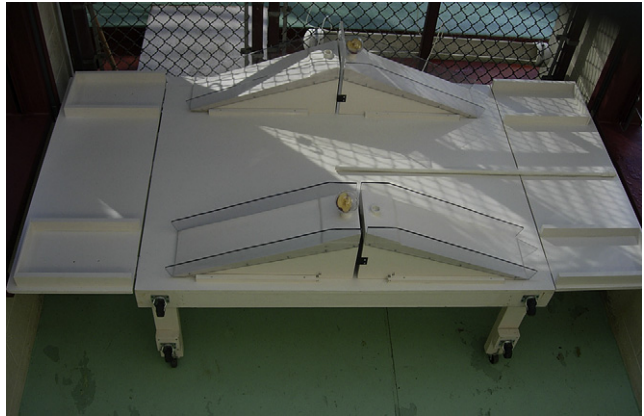
Figure 1. Experimental apparatus used in experiment 1. This figure does not show the black mesh barriers that divided the top of each ramp and that were used in all phases of the experiment. The mesh barriers replaced the clear Lexan barriers that are depicted here before testing began. When the capsule placed on the actor's side of the mesh barrier was dislodged, it rolled down the ramp towards the actor. When the reward on the recipient's side of the mesh barrier was dislodged through the mesh, it rolled down the ramp towards the opposite enclosure. The actor and recipient were 2.74 m apart and could see each other and the distribution of rewards.
